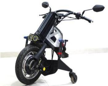
**NeoBolt** is a motor-powered clip-on which converts NeoFly into a safe, roadworthy vehicle. It eliminates the need to transfer into other vehicles and can be independently attached by the user within seconds. It has a maximum speed of 25 kmph and travels up to 30 km / charge. NeoBolt can be safely used on uneven terrains.
